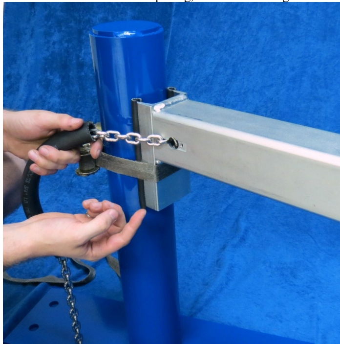
Figure 3. Chain is fed through circular opening, chain can be locked in by sliding into key-way.
