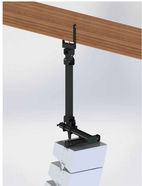
Figure 1. OFA-FL283-Kestrel Shown without optional top attachment hardware. Tilt is infinitely adjustable under full load.
