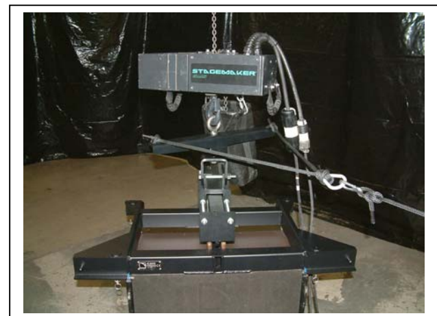
Figure 2. The Zbeam ® Lariat1100 attached to the SFA-16-1100 Spine Frame Adapter and Stagemaker ® electric chain hoist (sold separately), suspending an L-Acoustics ® DV-DOSC array.
